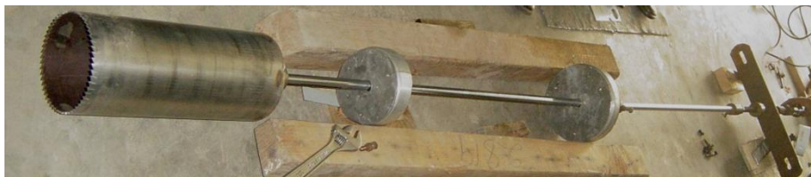
Fig. 5. The auger and associated fixtures.
