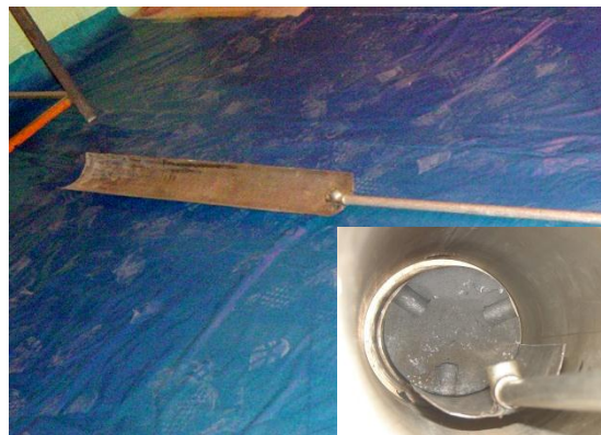
Fig. 4. Scoop used for graphite plug removal.
